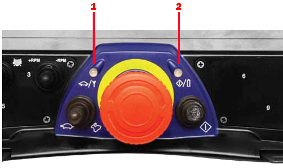
Figure 6.1 Status and alarm indication on portable control unit.
