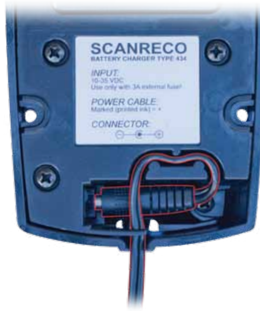
Figure 3.13 After connecting the cable connector; put the cable inside the cable track.
